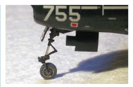
Bill cut the kit nose gear strut and added a new oleo and a set of styrene antitorque scissors.
